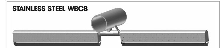
Our Stainless Steel WBCB diffusers are available in 304L or 316L stainless steel. The diffuser is made with cast endcaps welded all around. A typical piping system utilizing SSI WBCB diffusers is made from Stainless Steel pipe with 3/4" FNPT gusseted tees or elbows welded to the bottom center line.
